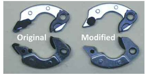
Left: A disassembled 009. Above: The original advance arms, left, and the modified arms at right. Below left: Top-down view of the original advancing plate.
