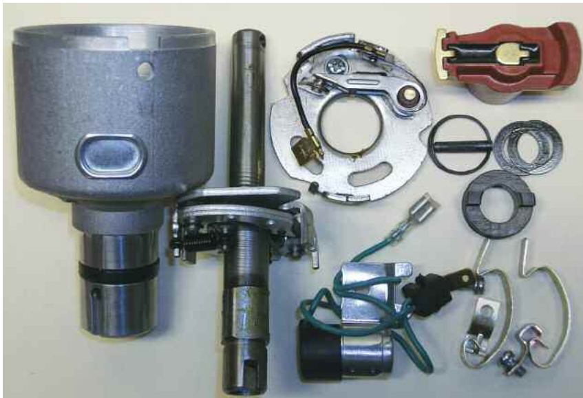
Left: A disassembled 009. Above: The original advance arms, left, and the modified arms at right. Below left: Top-down view of the original advancing plate.
