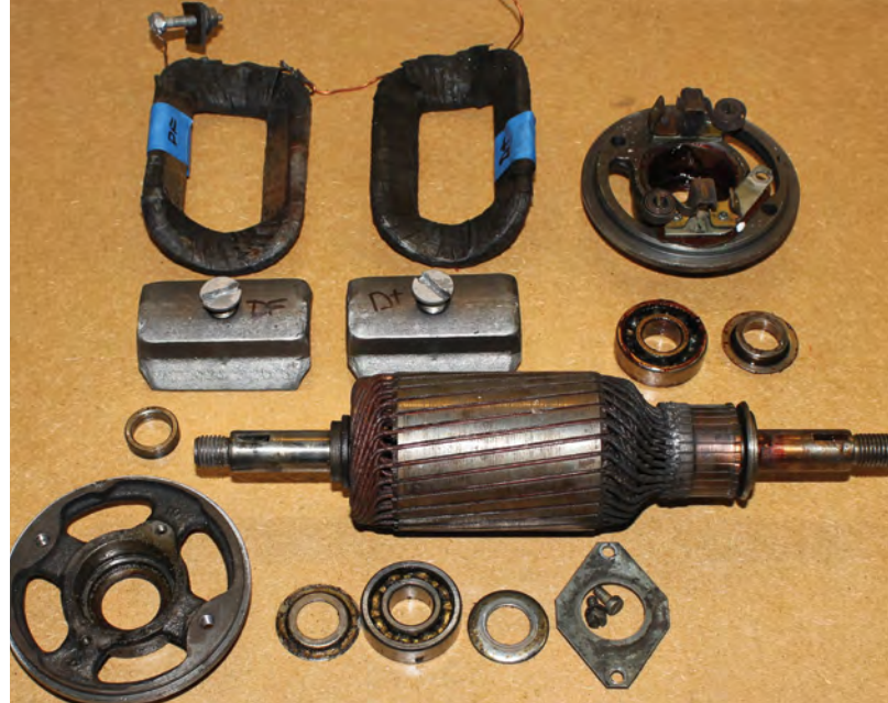
Fig. 5: The collection of disassembled Bosch generator parts. The field coil windings and pole shoes (top left) are labeled to guide reinstallation.
