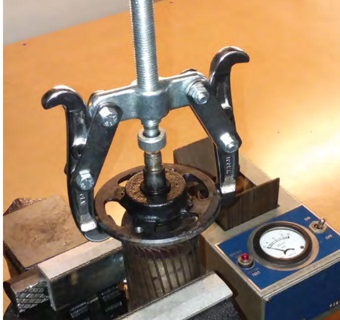
Fig. 3: The armature assembly and a two-jaw puller used for removing the end cover bearing housing. The device pictured next to the vise is the growler that will be later used to test the armature.
