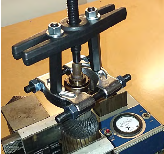
Fig. 4: The bearing at the commutator end is removed using a bearing separator and puller.
