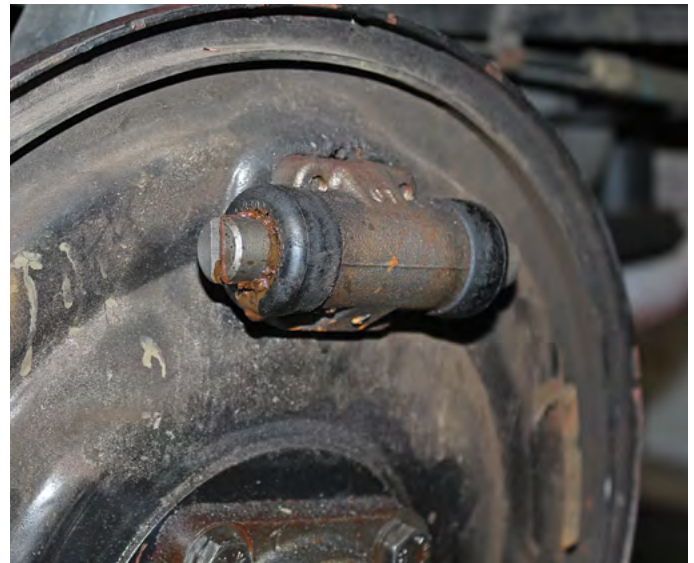
A rear brake cylinder with signs of leaking.
