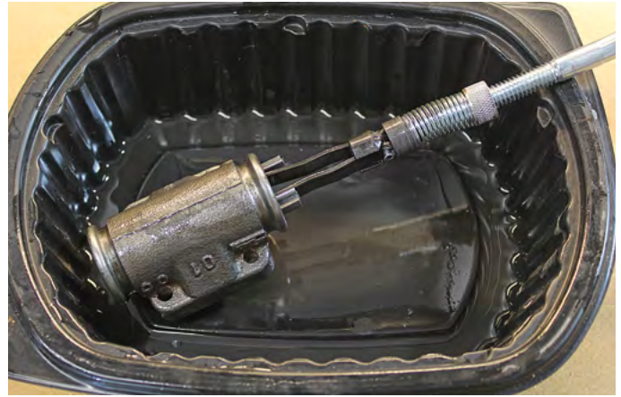
The brake cylinder hone inserted into a rear brake cylinder.
