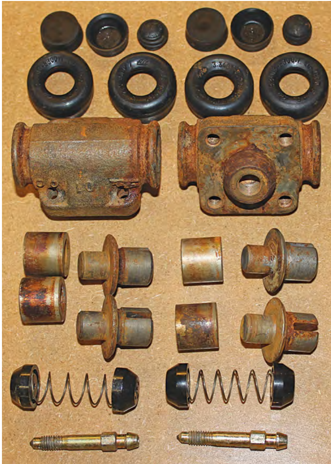
Disassembled rear-wheel cylinders and parts. The rubber cups and boots at the top will be replaced with new ones.
