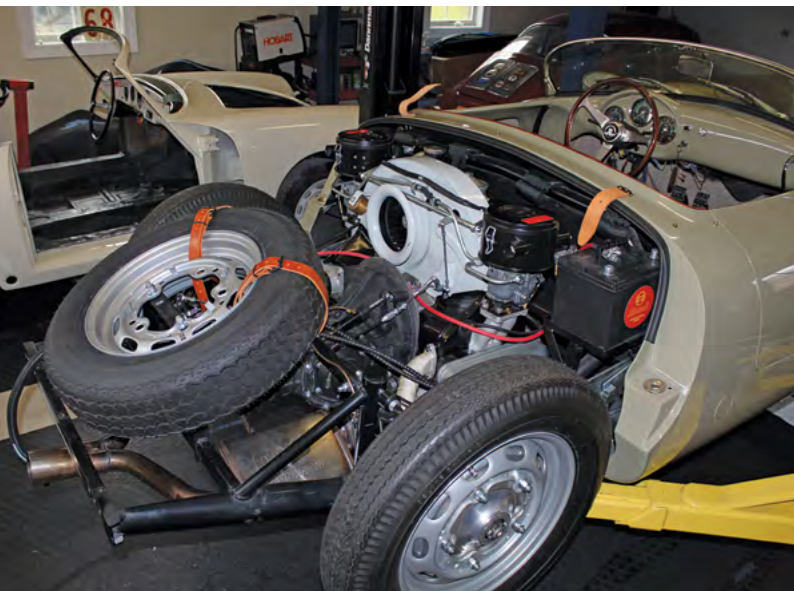
Motor mounted, custom fuel lines, cables, hydraulic lines, and wiring installed, ready for installation of the rear clamshell.
