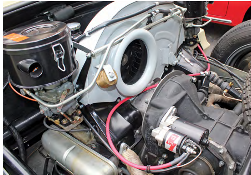
Twin-throated carburetors are seen in the specially-tuned 1500 Type 528 engine of one of the original early Porsche 550 Spyders (left, credit Porsche Spyders: Type 550 1953-1956 , Rodolfo Mailander, Ludvigsen Library Series, p. 11, 2002). My 616/15 motor is shown as installed in the Beck Spyder, with Zenith 32NDIX carburetors and 28mm venturis. Custom throttle cabling can be seen mated to the 356 throttle linkage (right).
