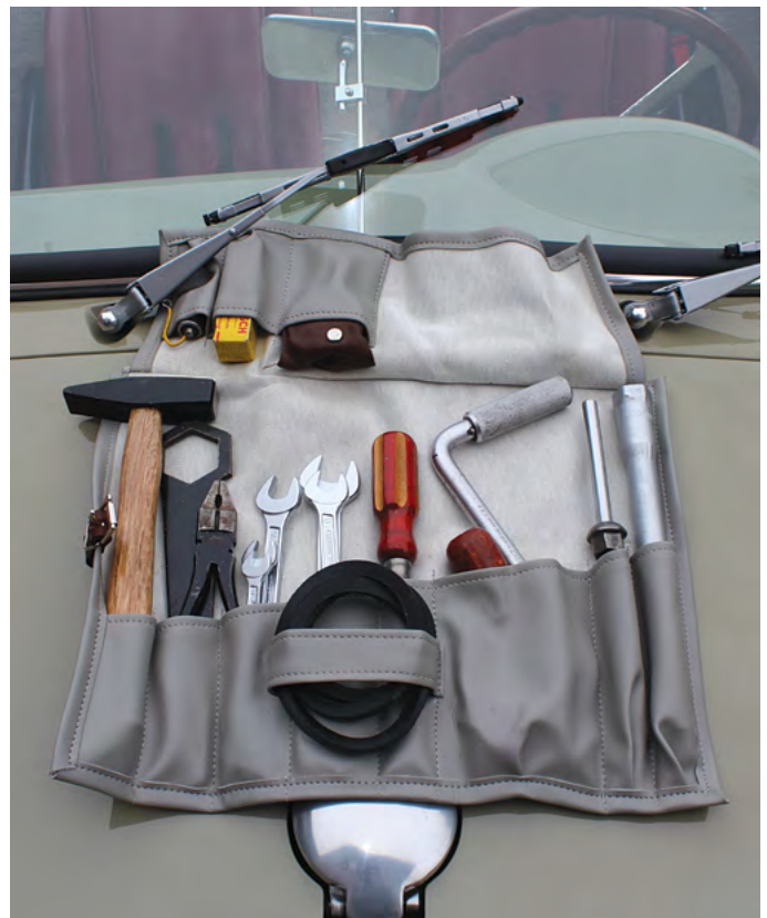
A toolkit based on the style and content of a '55, with some new and some old tools. The hardware and finish on the wiper arms were improved over those supplied with the car.
