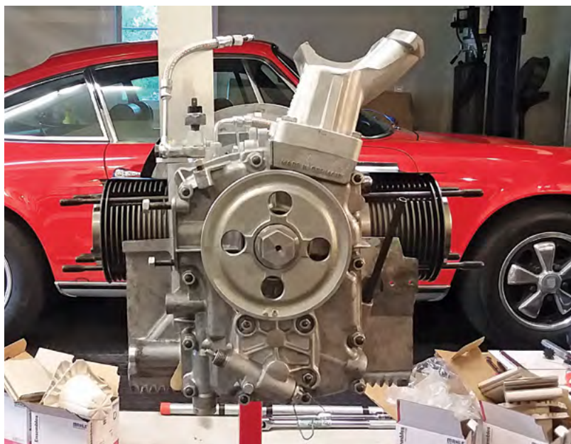
The 356C motor, after cleaning and machining, during assembly.
