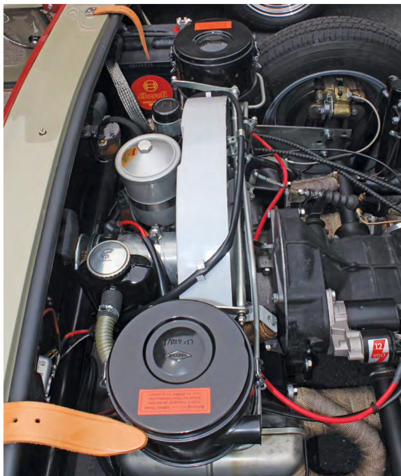
The C-style oil filler was cut down to allow the body clamshell to shut. The 12V voltage regulator and a glass bowl fuel filter were installed at the firewall. A new VW starter was used with the 12V, 200mm flywheel ring gear.
