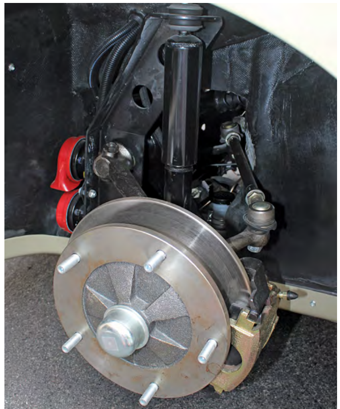
The ball-joint front beam and steering components are derived from the VW design, along with a shortened steering column. Front and rear rotors, calipers, and the brake master cylinder are parts from wide-five disc brake conversion kits.
