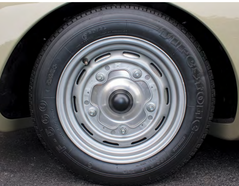
Firestone F-560 155R15 tires on 5 1/2 x 15-inch steel wheels. Wheels were media blasted, painted silver, and mounted over Fibersteel aluminum wheel skins at all four corners.
