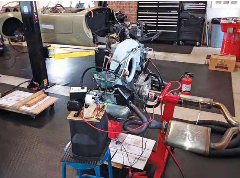
The Sebring exhaust mounted to the 616/15 motor, wired up for three-stage break-in on the test stand, during which I checked for leaks.
