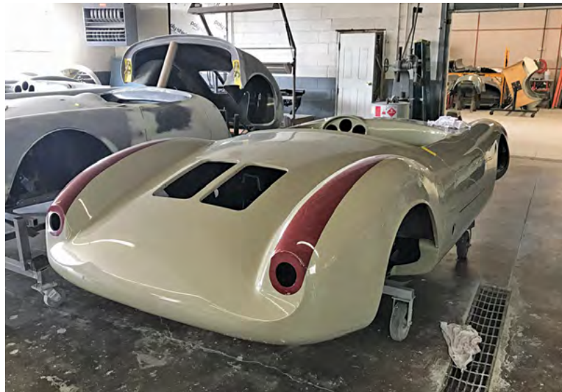
The Spyder body at Special Editions, after body work in primer (left) and after single-stage paint in classic Porsche 356 colors (right).
