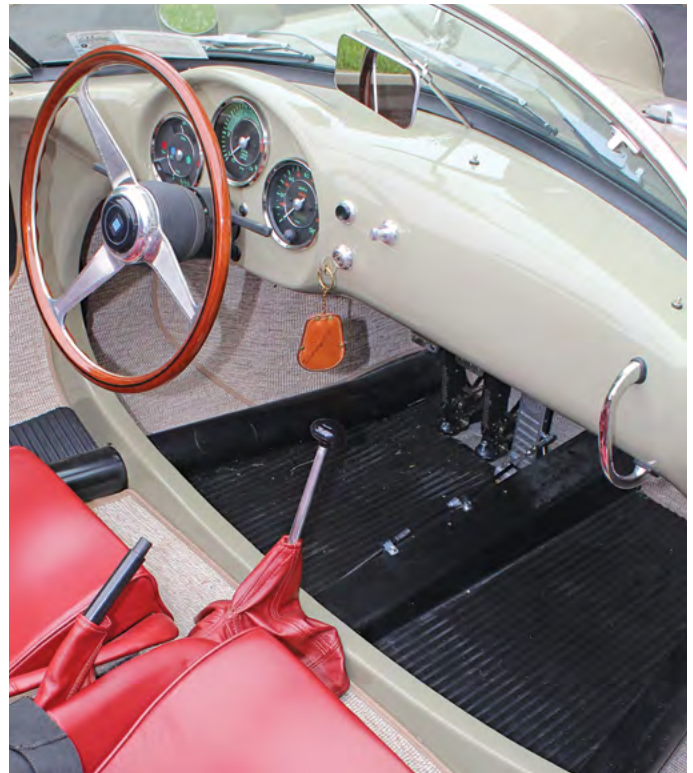
Dash instruments and controls in the original Porsche Type 550 Spyder (left, from the Porsche 550 owner's manual) and the Beck Spyder at right. Gauges in positions 3, 4, and 5 are new electronic VDOs, with GPS for the speedometer and odometer. Noticeably missing is the dual Autopulse electric fuel pump (14); I opted instead for the standard APG mechanical pump location at the motor. The steering wheel, pedal assembly (17, 18, 19), dash knobs (6, 8, 10), wipers, and footwell flooring were modified from those provided in the kit.
