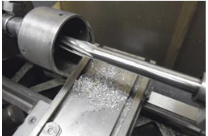
Drilling then reaming the bore of an older Bosch distributor to accommodate new bushings.
