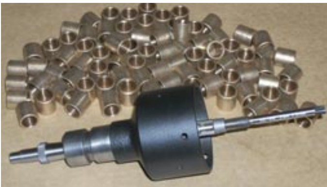
New modified plain sleeve bushings have been fit to this distributor and then hand reamed to size.
