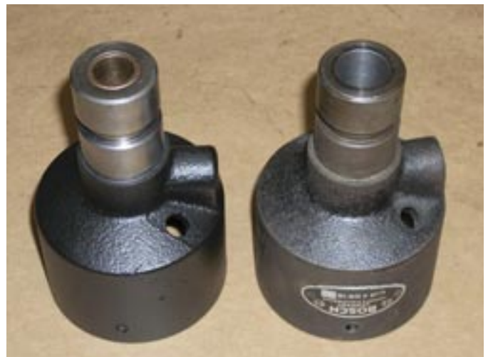
Two Bosch BR18 distributors bored to fit new bushings (right) and with bushings inserted (left).
