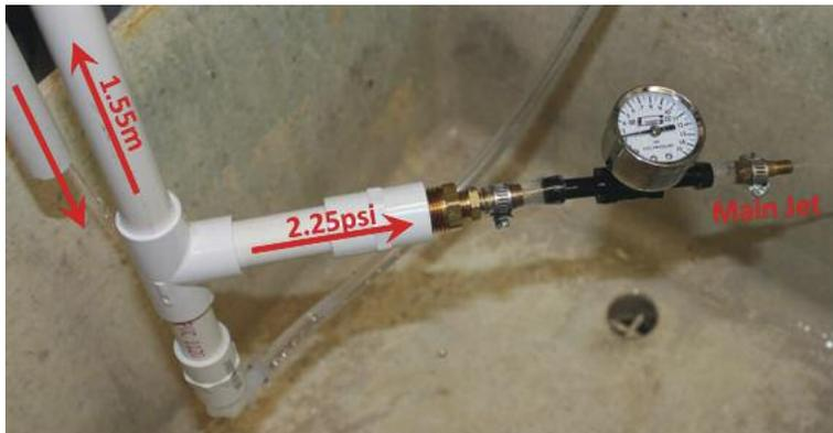
A 1.55 meter water column constructed to measure the flow rate through main jets. Water flows through the bottom of the column, up 1.55 meters past the 'head' to a vented u-fitting and drains off and down. The jet under test is at the end of the head and receives water at the constant relative pressure of 2.25 psi.
