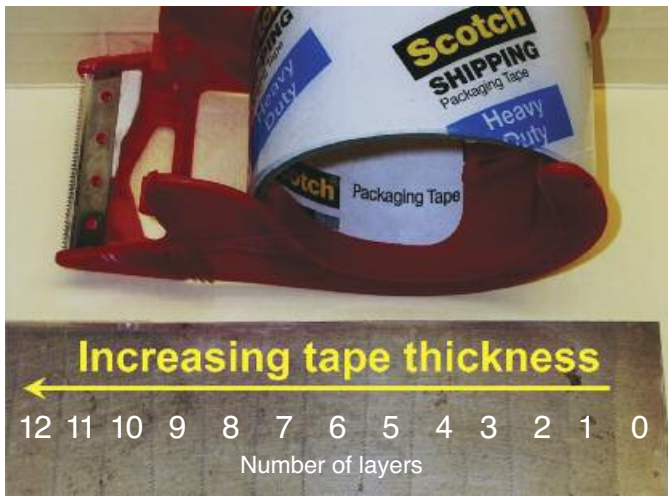
A calibration thickness standard using 3 mil polyester tape on steel.
