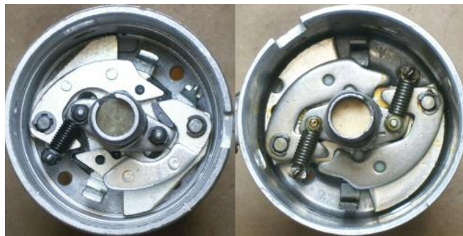
The straight line advance of Bosch 009 (left) and 050 (right) distributors are a result of spring tension countering centrifugal motion of weighted arms.
