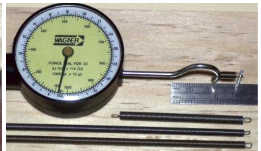
Commercially available stock springs (bottom) and the testing arrangement using a pull force gauge to measure and compare spring tension force.
