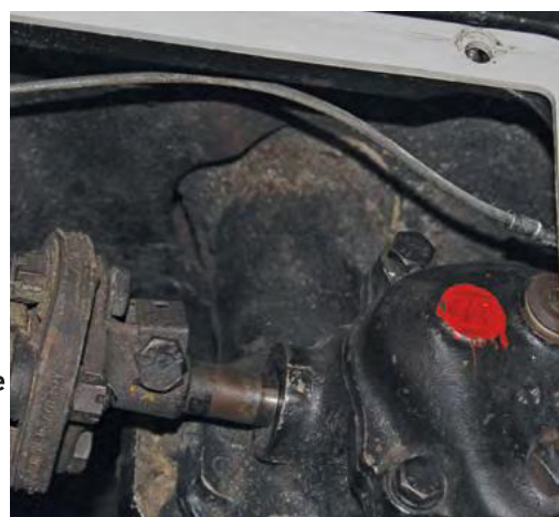
Fig. 13: With the block removed and the handbrake fully inserted, there should be some slack in the cable when it is disengaged. This allows for some pull of the handbrake handle before engaging the brake.
