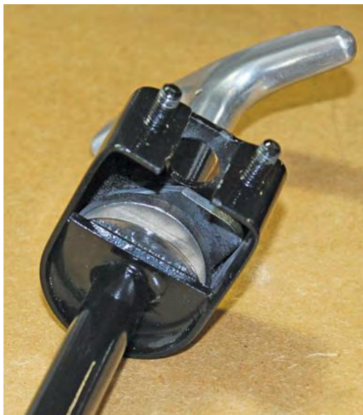
Fig. 9: Here are the parts in the unlocking position. The stop plate is now pointing to the left facing the handle, or to the right from the back side, and the bend in the locking plate is nearly horizontal.
