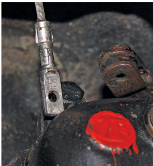
Fig. 11: This is the end of the cable as it meets the brake pivot. It will only fit into the receiver with a twist.
