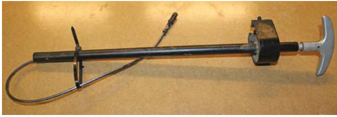
Fig. 4: The handbrake assembly removed from the car. The handle with cable is simply removed from the housing. The orientations of the locking parts should be noted before they are removed.
