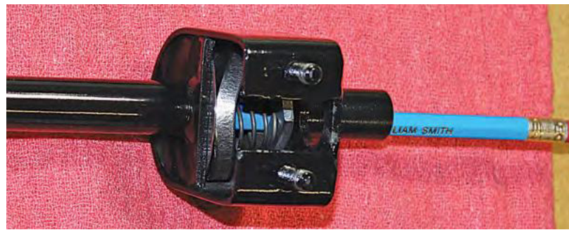
Fig. 7: Parts are being lined up in the housing prior to inserting the rod, using a pencil to keep them in place. Put the spring in after the other parts. Remove the pencil and feed the guide rod in while carefully aligning the parts.
