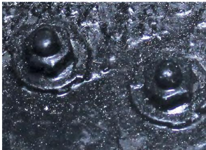
Fig. 2: The two M6 nuts holding the guide tube are found under the hood, next to the fuel tank.
