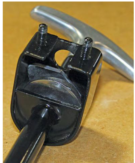
Fig. 8: Here is the orientation of the parts in the locked position, with the handle pointing at about 2 and 8 o'clock (facing the handle). The bend in the locking plate is vertical and the stop plate is pointing to the far right when facing the handle, or to the far left as pictured here from the backside.
