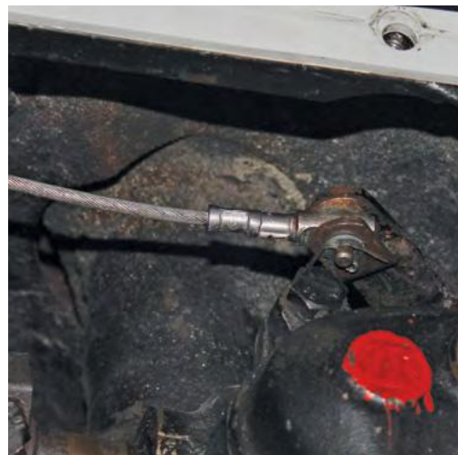
Fig. 12: Here is the cable inserted after twisting it a bit more than a quarter turn clockwise (viewed from the handle), with clevis and cotter pins inserted. The wooden block I mentioned in the text is still in place to keep the brake lever within reach.
