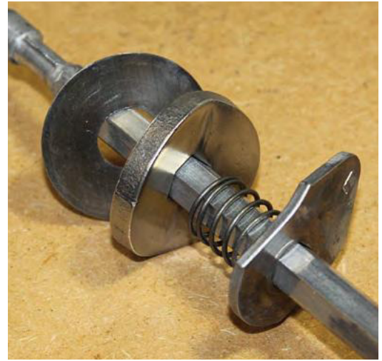
Fig. 6: This shows the order of the washer, locking plate, spring, and stop plate on the hexagonal rod outside of the housing. To assemble, the locking parts should be placed in the housing before inserting the rod and cable.
