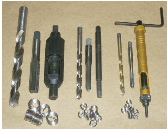
Three helical insert sets for thread repair: M12x1.25mm for carburetor fuel ports (left), M7x1mm for jet cover bolts (center) and M5x0.90mm for Zenith cover top screws (right).
