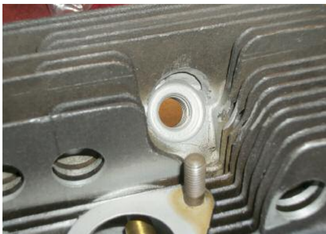
Spark plug holes in our 356/912 motors use threaded coil inserts from the factory.
