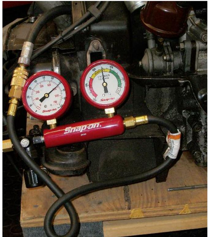
A dual gauge leak-down tester is connected to cylinder #4 and the crank is set to its corresponding TDC. Once the pressure is set to zero out the right gauge, it is connected to the cylinder under test to read leakage. A leak at the intake valve seat is the reason for this cylinder's 50% reading.
