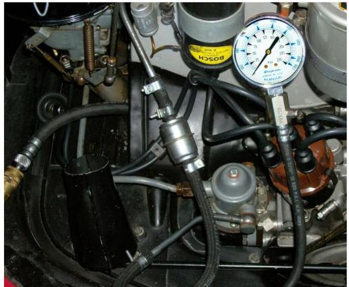
A compression test gauge is connected to the #4 cylinder, which is ready to test. The engine has been warmed up and plugs removed. With the carb throttle plates open, the engine is cranked over several strokes until max pressure is reached.
