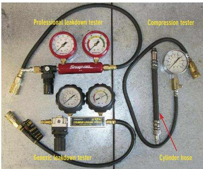
A pair of dual gauge leak-down testers (left) and a compression tester (right). The cylinder hose is used to connect to the cylinder under test by threading it into the spark plug hole. The quick-disconnect style hose fitting makes for easier threading.
