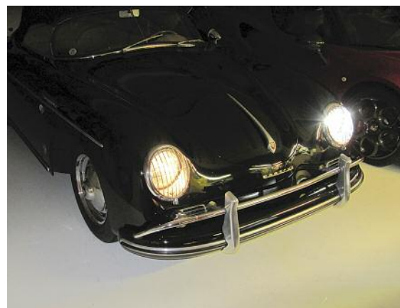
The LED headlight appears clearly brighter in this photo with one original incandescent bulb still installed. One caveat to "eyeball" measurement is the fact that higher color temperature (toward the blue cast) gives a psychological impression of brightness.
