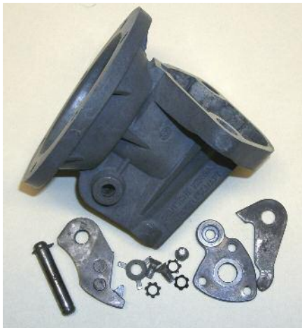
VW fuel pump parts, including the base, that can be used in Porsche A/B pumps.
