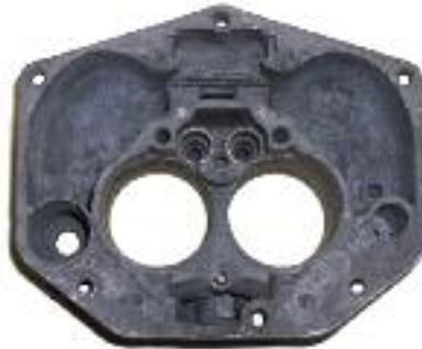
Above: After brushing with a brass wire brush, a successfully cleaned Zenith carburetor body - inside and out. Left: Too long in less than optimum conditions.
